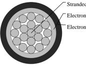
Stranded Tinned Copper Conductor Electron Beam Cross-linked Insulation Electron Beam Cross-linked Sheath
